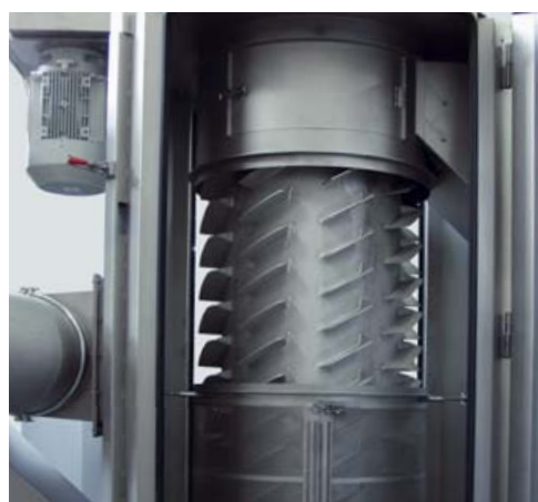
Rotor and sieve inside the CENTRO centrifugal dryer
