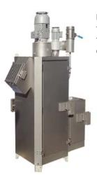
Integration of the intake and air filter into the resin outlet optimizes countercurrent air flow so less air volume is needed for the drying process.
