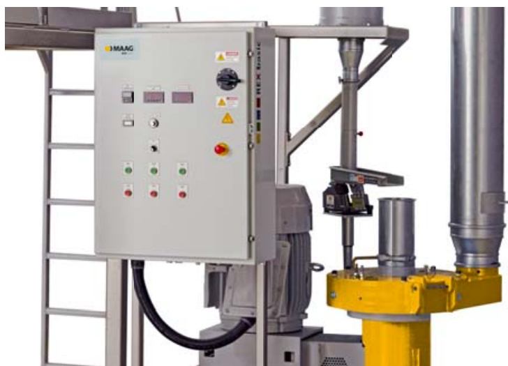
Mill Chamber and Manual Controls
