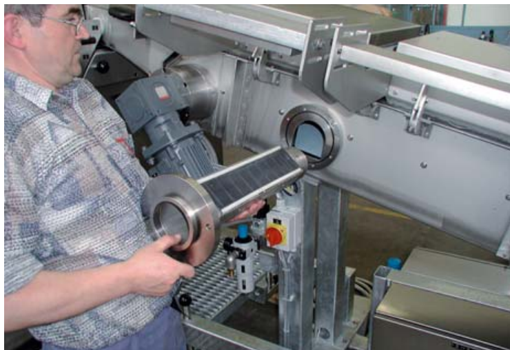
Variable positioning of the exhaust air nozzles
