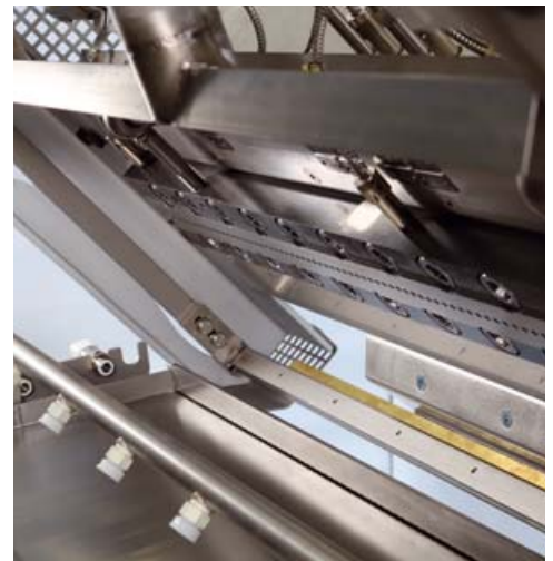
JSG 900 start-up device with scraper and HAK
