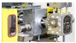
Maag system with extrusion pump and arched screen changer
