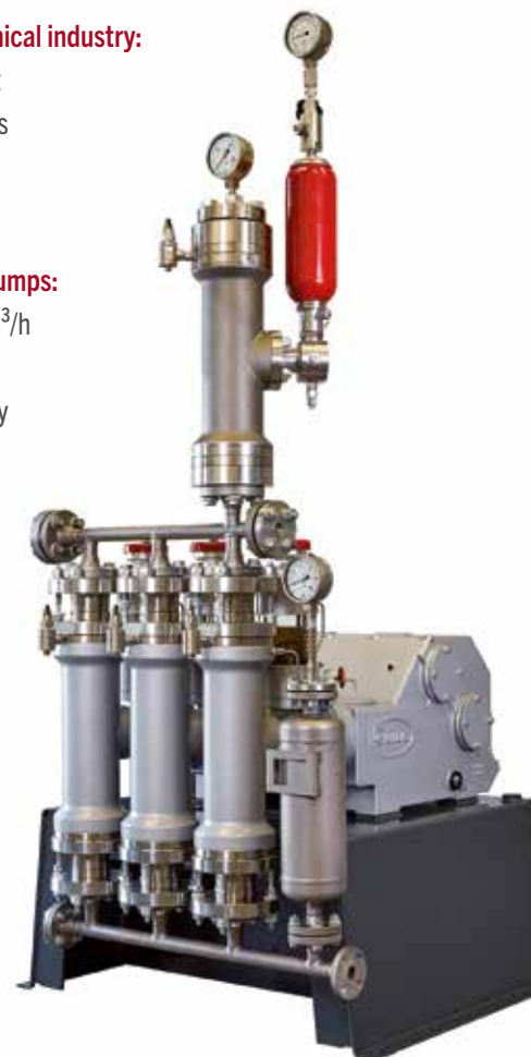
MULTISAFE® double hose-diaphragm pump Flow rate: 2.1 m 3 /h Pressure: 60 bar Conveyed medium: polyaluminium chloride Special feature: titanium piping
