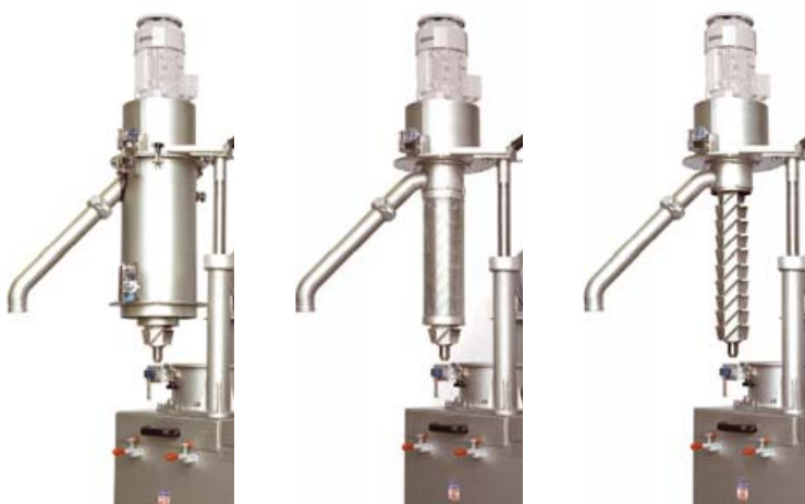
Left to Right: Model 1150 Dryer housing, screen assembly and rotor
