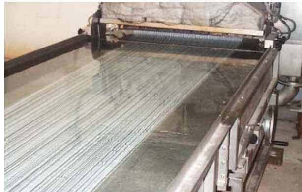
KW 1.400 cooling trough for up to 130 strands
