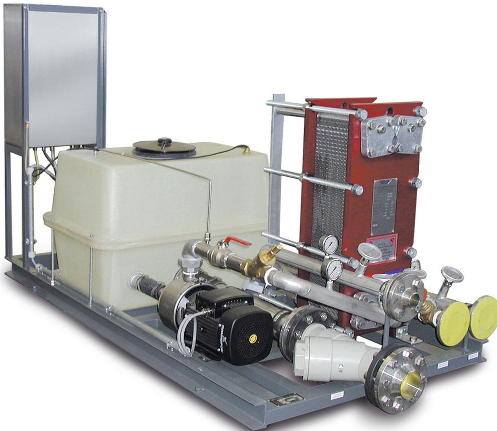
The process water treatment unit PWA serves for filtering, tempering, and circulating the process water in compound and masterbatch production and can be integrated into the base frame of the cooling trough or positioned externally. Using a heat exchanger, the PWA separates the contaminated process water circuit from the primary cooling circuit from the central water supply.
