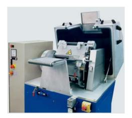
The Rotor is a replaceable segment, milling type helical design. Rotors are available in a variety of materials. Tool steels, stellite tipped, and contamination-free, carbide tipped specific designs are dependent on the cutting application.
